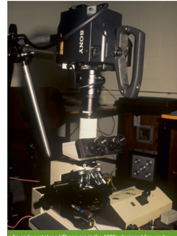
An early prototype HD camera in the 1990s designed for use by surgeons, bolted onto my microscope as an experiment at Sony Professional Solutions Europe, Basingstoke
