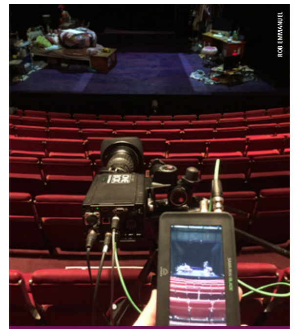
Locked-off P70 camera on a Manfrotto stills tripod – a wide of the stage in portrait really doesn't work and it was impossible to avoid shooting multiple seats foreground
