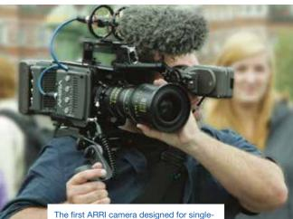
user operation: here with optional handgrip and Fujinon Alura 30-80mm PL zoom lens
