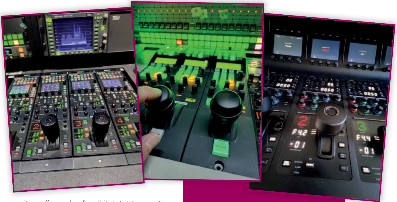
A trio of remote control panels, from left to right: Sony RCP-1550, Grass Valley OCP-400 and Blackmagic Design Advanced Camera Control Unit
